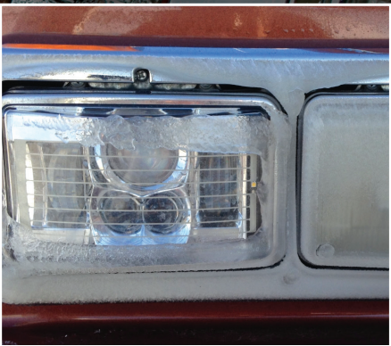
Automatically de-ices headlight according to ambient temperature
